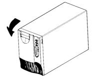
2. Slide up and remove the metal battery cover.
